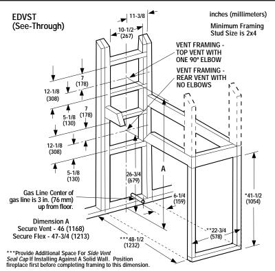
\*\*This dimension based on 5/8" drywall. For 1/2" drywall use 23"
