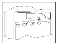
Figure 2a - Top Baffle Removal
