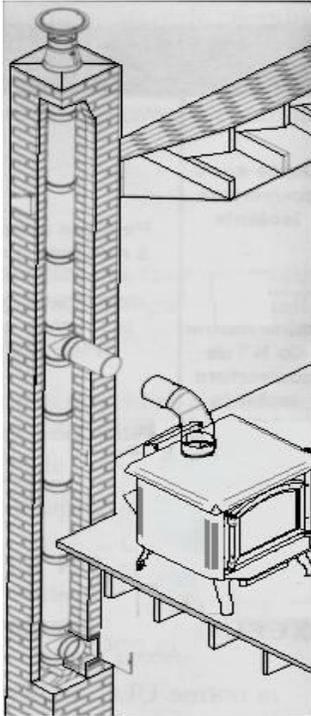
The *Tison* and *Cuisiniere* models must be installed in accordance with the applicable local laws or the CAN/CSA - B365 ULC S635, ULC S640 standards. For the chimney, follow the chimney manufacturer's instructions.
