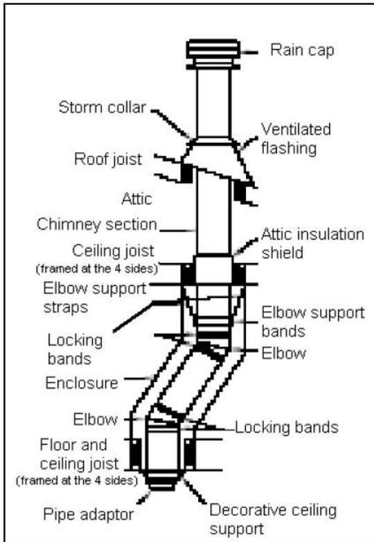
The *Tison* and *Cuisiniere* models must be installed in accordance with the applicable local laws or the CAN/CSA - B365 ULC S635, ULC S640 standards. For the chimney, follow the chimney manufacturer's instructions.
