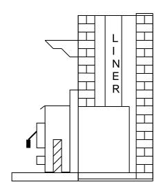
8 inch chimney liner. If the floor of the fireplace is recessed below the hearth build up floor with steel shims, firebricks, or another noncombustible material to hearth level so the insert sets level. Insert this liner in the chimney now and support up in chimney until your insert is in place. Now position your insert on the hearth.
