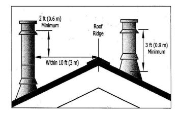
**Chimney Draft Requirements:** Chimney draft is the measurement of the pull or vacuum created by the chimney. It can be measured with a manometer and is expressed in inches of water (kPa). To measure you need to drill a small hole in the stovepipe between the flue collar and any stovepipe dampers installed into the stovepipe system. Insert the manometer connection into the hole and note
