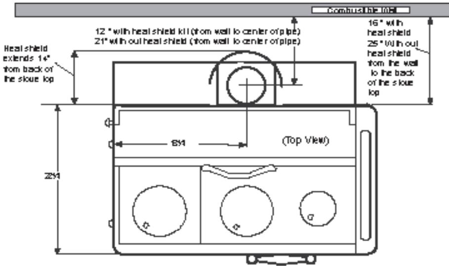
These drawings are for reference only, showing approximate dimensions for rough in purposes. Make sure that no floor or ceiling supports will be cut due to chimney installation.
