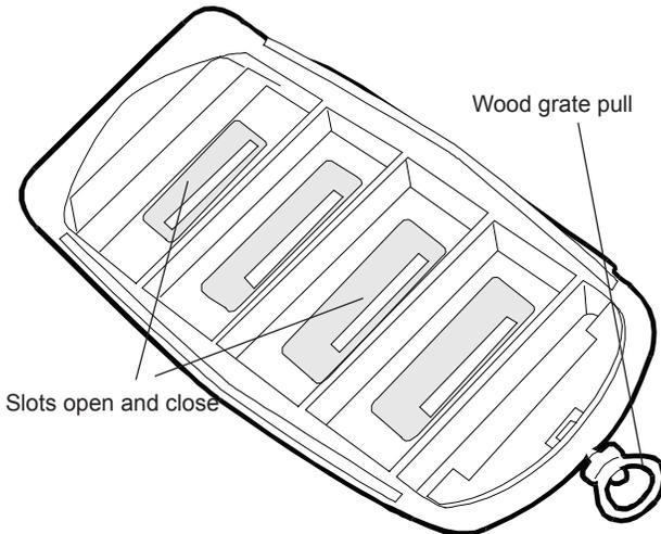
The stove is burned with the slots open which allows the combustion air to enter underneath the fire. As ash and coals build up on the grate these slots fill and will require the occasional "shaking".
