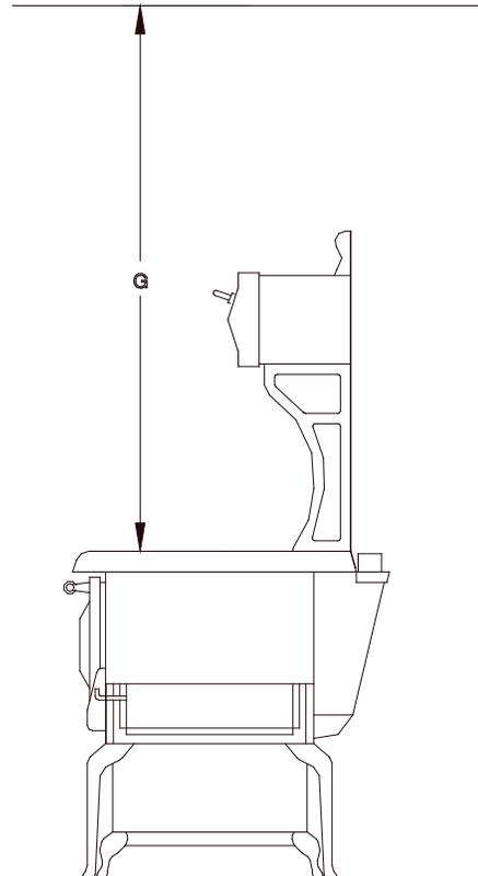
When a heat shield is installed dimensions B, D, E and F are taken from the heat shield. Dimensions A, C, G, and H remain the same with or without a heat shield. Dimensions A and C are taken from the *reservoir* on reservoir models. When two or more clearances to combustible walls contradict each other, the clearance with the greater numerical value must be maintained.
