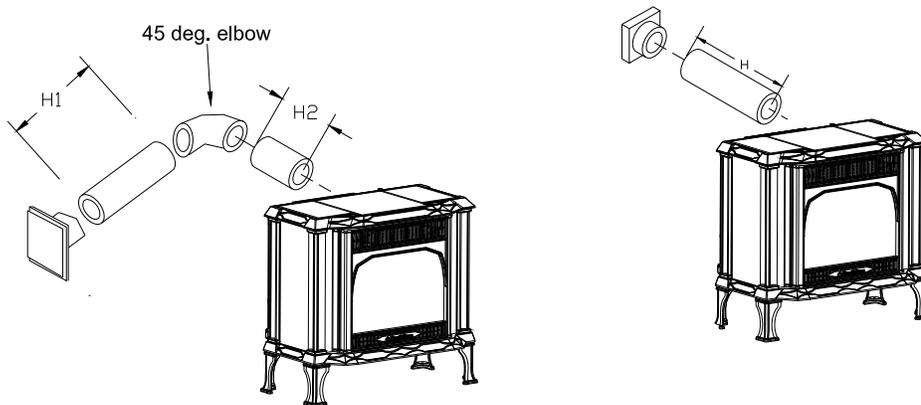
CENTERLINE OF PIPE IS 21.25" ABOVE THE FLOOR
