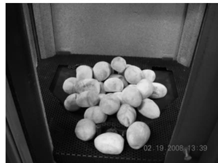
4. Install 10 stones on the second layer, filling in spaces in the lower level. Distribute the stones evenly over the burner. NEVER stack the stones more than 2 high
