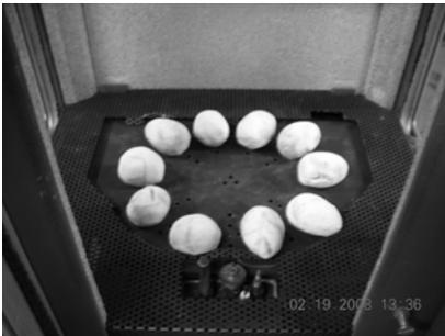
1. Install 10 stones in a circle pattern. The stones must not cover the burner ports of the outer ring on the burner, and should fit in between the burner ports.
