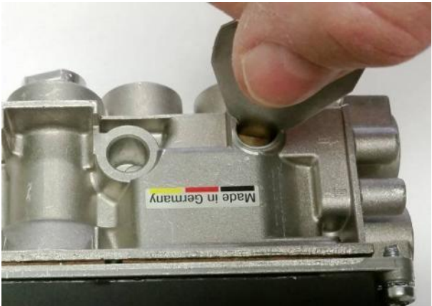
Figure 25 – Tighten LP Low Flow Orifice
