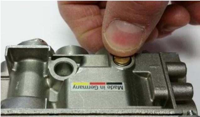
Figure 23 – NG Low Flow Screw Removal
