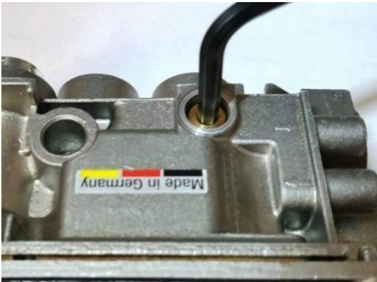
Figure 21 – Low Flow Orifice Removal
