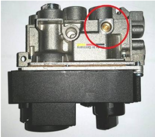
Figure 20 – Low Flow Orifice Location
