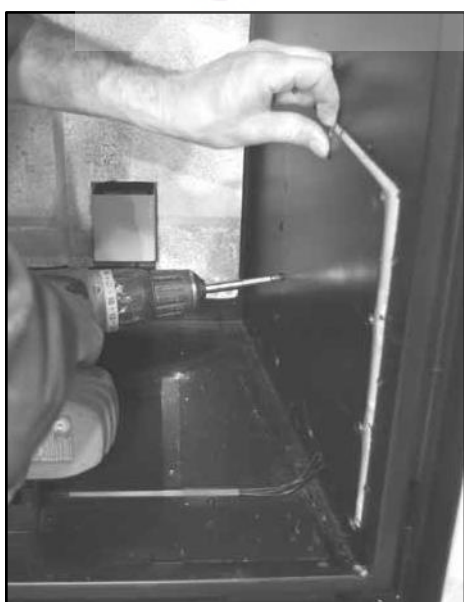
Figure 13: Removing Access Cover.
