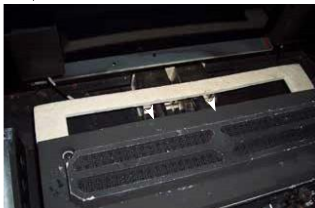
Figure 65: Move Burner away from Mixing Tubes
