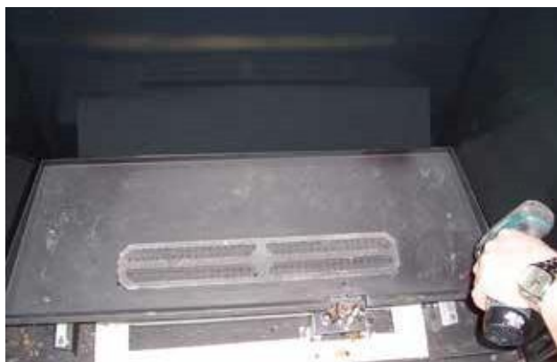
Figure 64: Burner Screw Locations
