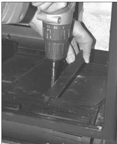
Figure 56: Removing the Right Burner Support.
