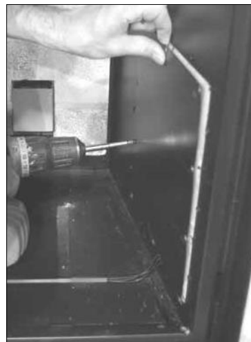
Figure 57: Removing Access Cover.
