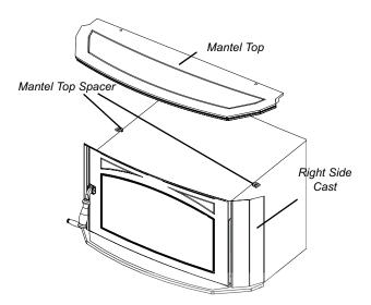
With the Mantel Top in place check to make sure there is no gap between the Mantel Top Spacer and the underside cast of the Mantel Top. If there is a gap present you will need to lower that side cast by loosening 2 bolts, see side cast adjustment section for bolt location (check to see if level).
