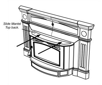
Adjust Left Side Faceplate and tighten bolts. Repeat step for Right Side Faceplate.
