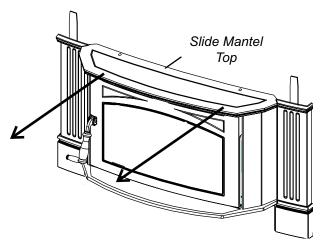
5) Mount the Top Faceplate by carefully sliding the Mounting Plates on the Left and Right Side Faceplate thru the Retainers in the Top Faceplate.
