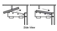
Tilt the left baffle up on top of the side channel and it will leave enough room to position the right baffle in the same manner as Step 1) above. Then reposition the left baffle flat on the air tubes.
