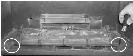
Remove the 2 screws, push Burner Assembly to the left and lift out.
