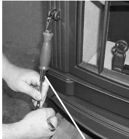
Secure using 7/16" socket wrench.
