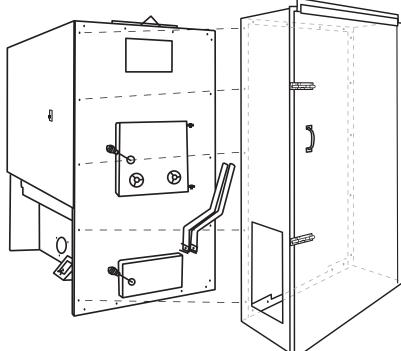
Use 18 - #14 x 3/4 self tapping screws to attach O.F.D. to front of furnace.
