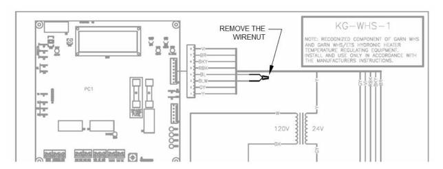
2.) Connect the BLUE/BLUE-WHITE wire pair to either side of a dry contact provided by the utility. The contact is closed when off-peak is available and open when off-peak is not available.
