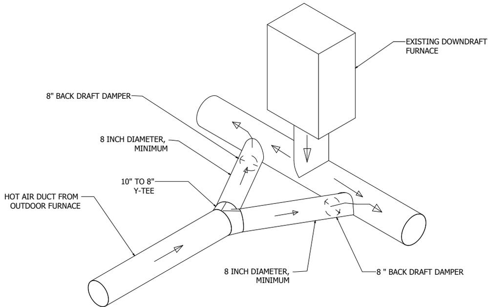
**NO DUCT WORK INSTALLATION CONNECTION:**
