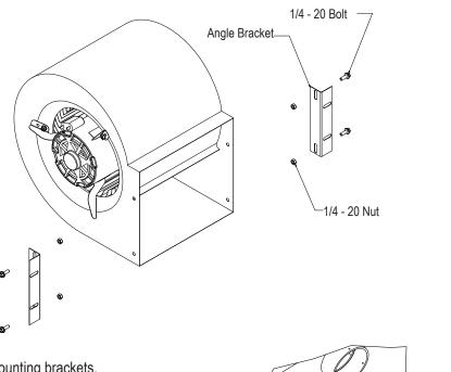
2. Attach blower to the left and right mounting brackets.
