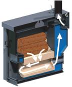
maintains burn chamber temperatures for consistent combustion. This high temperature gasification significantly lowers emissions, prevents creosote buildup and minimizes ash buildup in the furnace. After passing through the burn chamber, exhaust air is forced through multiple flues running through the water jacket, heating the water quickly and efficiently.
