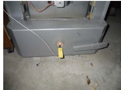
“K” type thermocouple measuring secondary chamber temperatures
