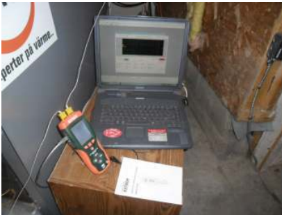
Data logging chimney smoke and secondary chamber temperatures using “K” type, high temp. thermocouples
