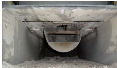
Fully water jacketed secondary chamber with stainless steel afterburner
