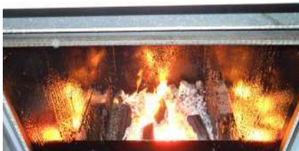
Fire in primary chamber – the vertical walls are wider at bottom than at top to reduce wood fuel “bridging”
