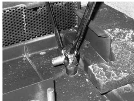
Burner Orifice Removal
