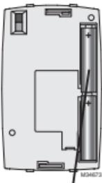
Turn thermostat over, insert fresh AAA alkaline batteries, then reinstall thermostat.
