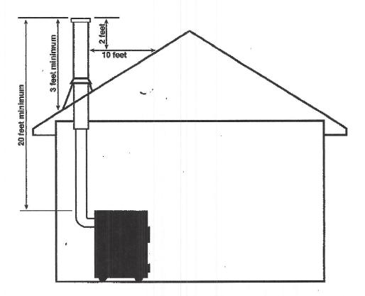
According to NFPA Standards single wall stove pipe can be within 9" of combustible provided an approved fire retardant material covered with 28 gauge sheet metal, spaced out 1" on non-combustible spacers is utilized.
