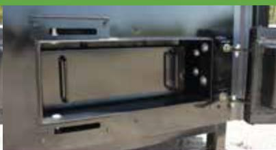
Secondary Combustion Chamber Heat Shield
