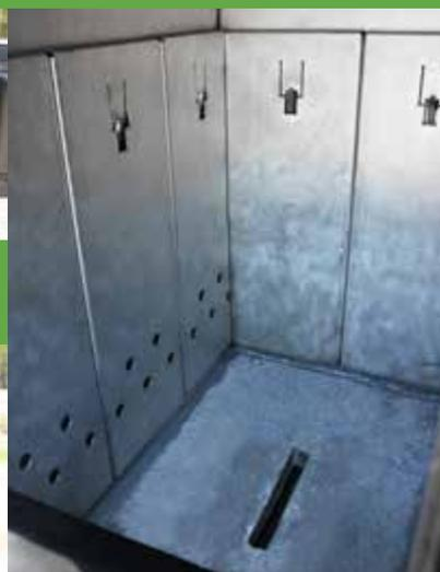
Air Panels & Gasification Manifold
