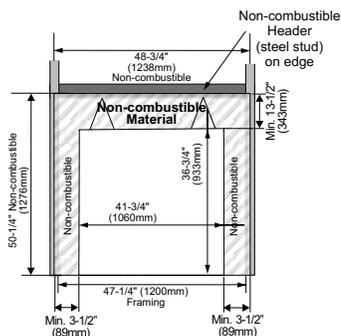
**\*\* Important: Framing height requires consideration of the hearth depth. Dimension N = N + the thickness of the installed hearth.**
