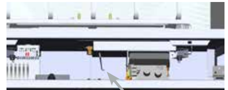
Air shutter rod: located to the left of the valve assembly.
