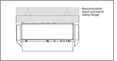
Figure 42: Noncombustible Material with Surround— Profile View
