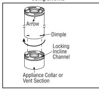
Figure 18: Connected vent components
