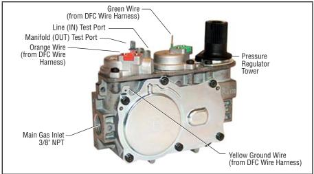
The SIT gas valve in this fireplace has a 3/8" NPT thread main gas inlet and outlet. Test gauge connections are provided on the front of the electronic gas control valve (identified IN for the inlet and OUT for the manifold side).
