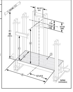
Table 11: Fireplace Framing Specifications—Corner Installation with Horizontal Termination
