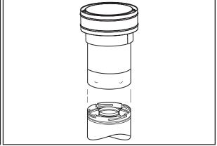
**12. Install the vertical termination**—Extend the vent sections to the correct height (*Figure 4*). The SV4.5CGV-1 Vertical Termination (*Figure 24*) installs in the exact same fashion as any other Secure Vent® section.
