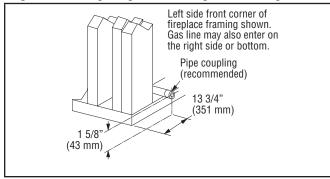
Figure 10: Routing the gas line into the fireplace
