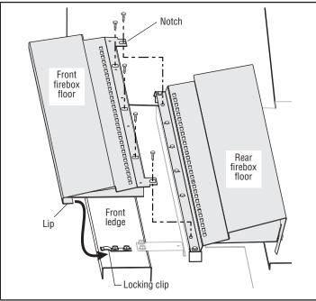
Installing the rear firebox floor
