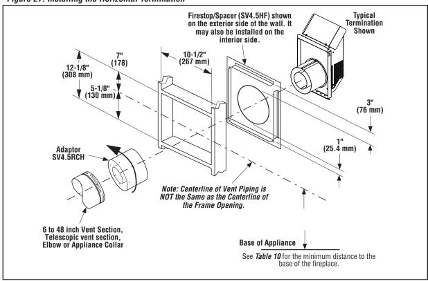
**NOTE:** To help minimize water infiltration install the firestop/spacer (SV4.5HF) on the exterior side of the wall.
