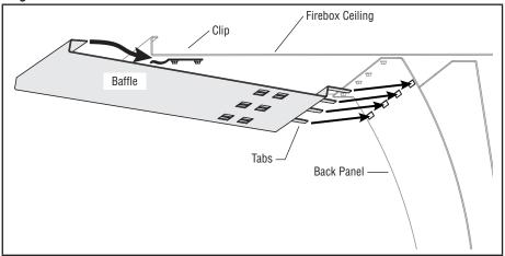
2. While sliding the tabs into the slots, slide the front lip of the baffle under the clips in the firebox ceiling.
