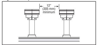
Terminate single vent caps relative to building components according to *Table 6* and *Figure 4*.
