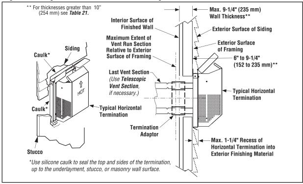
Table 21: Venting Components Required for Various Exterior Wall Thicknesses, when using Typical Termination Kits
