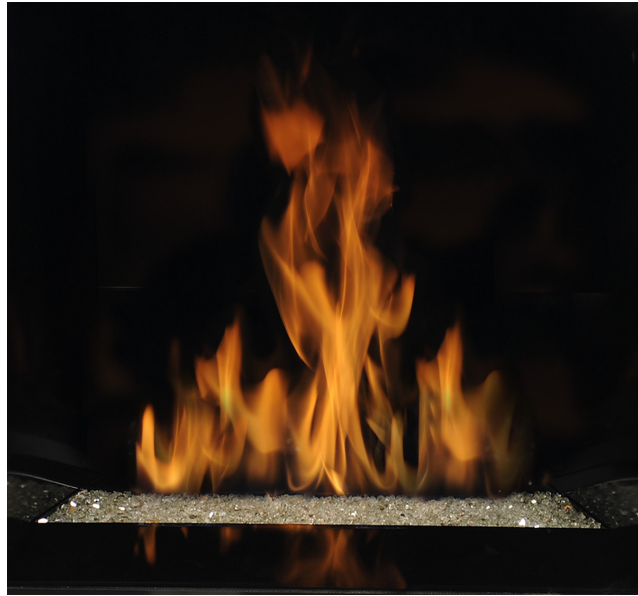
Figure 18 - Burner Flame Appearance
