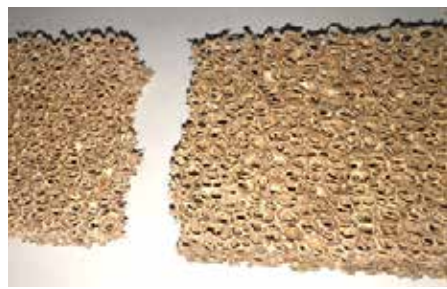
Combustor Problem - Broken Combustor
