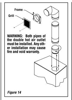
When installing the double outlet system, the hot air outlets can be installed in the same room as the fireplace, or one or both of the outlets can be installed in adjacent or upper rooms. Installing the ducts at different elevations will tend to exhaust more heat out of the higher outlet (*Figure 15*).
