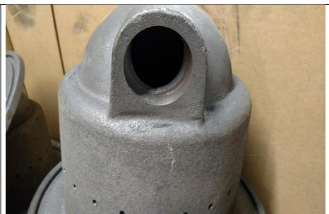
Step 7: Test fit the auger tube into the new burn pot. Be sure the tube mates against the inner surface of the pot. Remove the tube after test fitting.
