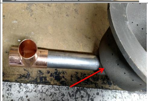
Step 8: Turn your burn pot upside down and notice there is a groove in the casting of the pot. This groove fits onto the edge of the burn pot holding ring. Using a High-Temp liquid stove gasket cement (we recommend Rutland name brand) liberally fill the groove with the gasket cement. The gasket cement can be purchased at most hardware stores or directly from LMF Mfg.
