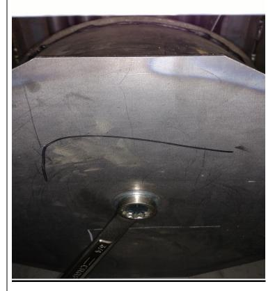
inside to feel the head of the bolt. Remove the bolt and washer. There is a new bolt and washer supplied with your new Pot.
