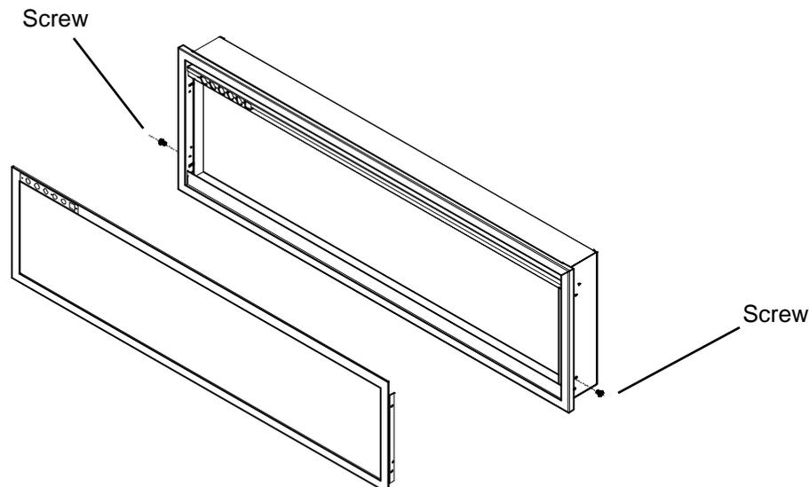
2. Unscrew the 2 screws located on each side and take off the inner side steel panels.
