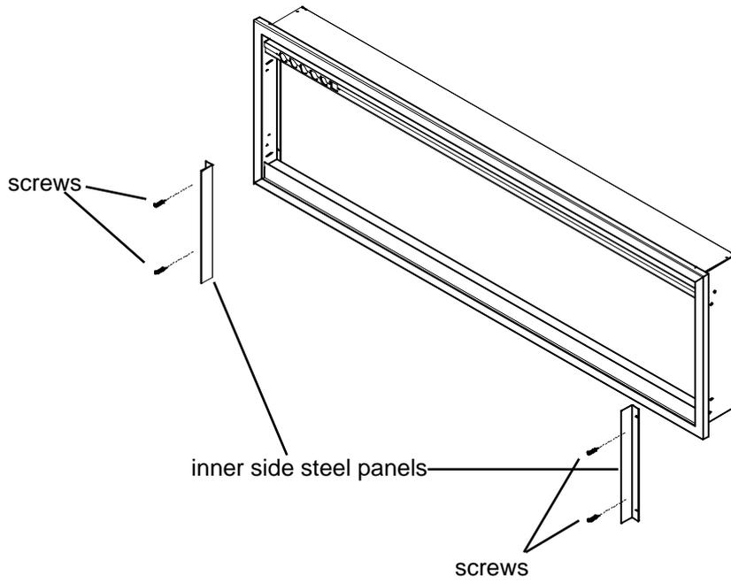
3. Put the fireplace into the wall opening and fix it to be the wall.
