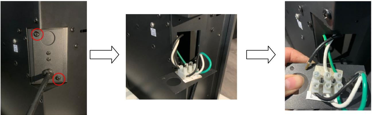
2. Cut off the copper head of the wiring and leave 1 cm (0.4 inch) uncovered wiring.
