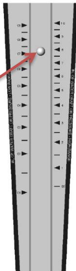
**Unhealthy flue:** The flue draught meter shows a reading well below the required operating range that will result in poor, smokey performance.
