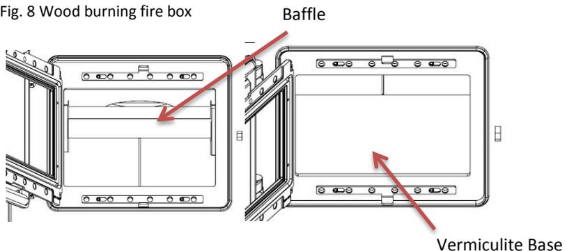
To set the cooker back into a wood burning configuration, remove the grate, ashpan, ashpan support plate and reinstate vermiculite base bricks, catalysers, catalyser bracket and gasket as shown in Figure 4.
