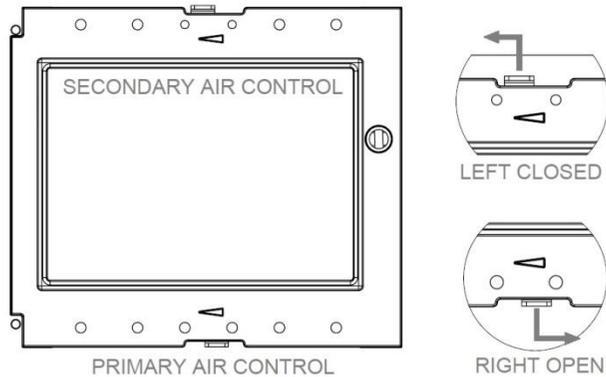
Fire door closed, with primary and secondary air sliders in the open position to the right hand side.
