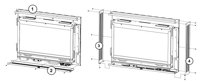
Secure the housing panels as illustrated using the 17 #8 X 3/8" screws supplied.
