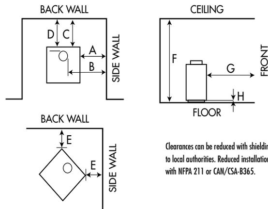
Clearances can be reduced with shielding acceptable to local authorities. Reduced installation must comply with NFPA 211 or CAN/CSA-B365.
