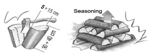
The logs are kept chopped and arranged. After their seasoning in summer under the influence of the sunbeams and the warm air their dampness must fall under 20%. A dry piece of wood is cracked in his edges. The thickness of the logs must be between 5 and 15 m.
