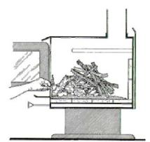
The aim is to kindle the fireplace with one stick of matches, without unnecessary fuss and repeatedly adding of paper and kindlings.
