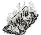
kindling occurs with a sufficiently high temperature and the presence of air maintaining the burning. The gases burn with bright flames. When no kindling occurs, the smoke either condenses on the pipes and the chimney in a shape of tarry precipitations or it is thrown away, polluting the environment. The non-kindled smoke carries away the bigger part of the energy containing in the logs without any use.
