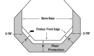
The floor protection must be a non-combustible material extending beneath the stove and to the front and sides as
