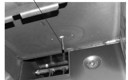
Fig. 119 Cleaning the thermocontrol sensor
