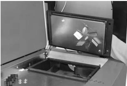
Fig. 129 Unscrewing blower unit
