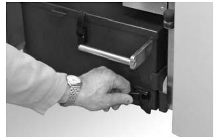
Fig. 113 Opening the bracket fastener
