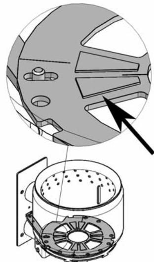
Fig. 124 BioWIN 210/260, Grate plate with embossing pointing upwards
