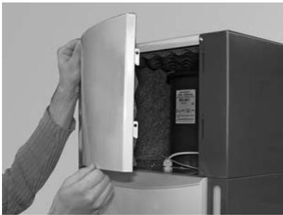
Fig. 134 Removing the cladding
