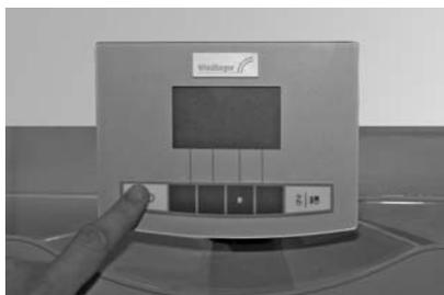
Fig. 117 Switching off BioWIN
