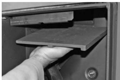
Fig. 118 Cleaning the baffle plate
