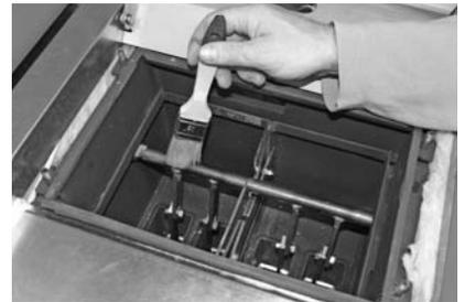
Fig. 131 Cleaning the coating surfaces
