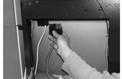
Fig. 128 Disconnecting the blower plug
