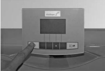
Fig. 126 Switching off BioWIN
