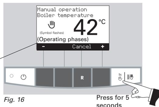
Pressing the *Cancel* button or *Manual operation / chimney sweeper function* button terminates the function – Fig. 22. The boiler returns to automatic operation.
