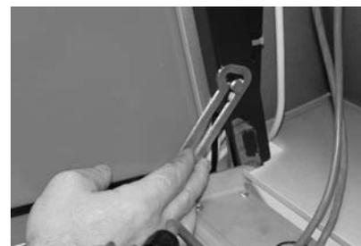
Fig. 133 Loosening locking arm
