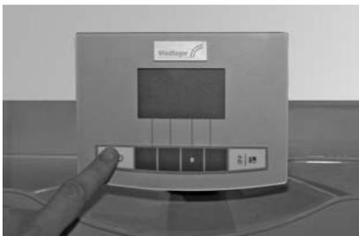
Fig. 108 Switching off BioWIN
