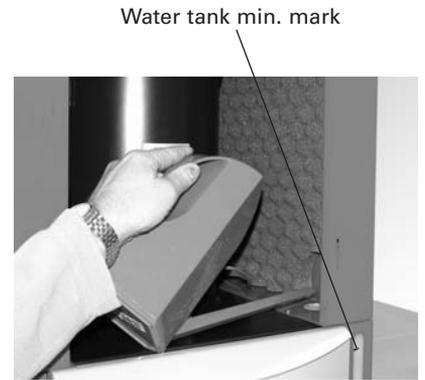
Fig. 136 Filling water container
