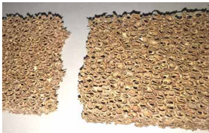
Combustor Problem - Broken Combustor
