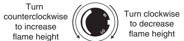
Fig. 30 Flame adjustment knob for SIT valve.
