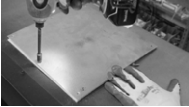
Step 1: Remove the two (2) screws holding the top vent cover plate and gasket.
