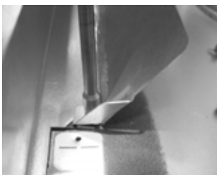
Step 2: Secure all three of the screws to the up-right positioned heat shield - one (1) at both ends and one (1) in the center.
