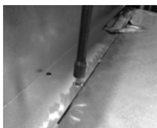
Step 2: Secure all three of the screws to the up-right positioned heat shield - one (1) at both ends and one (1) in the center.
