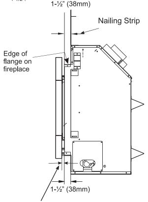
**Important:** 1/2" gap required between faceplate and finished wall when using part #316-924, 316-926, 316-927 (4 pc. faceplate).
