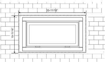
6) If finishing the unit with the inner faceplate only - the finishing material may be brought up to the edge of the unit.
