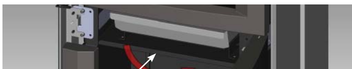
Ashlip to be positioned here
