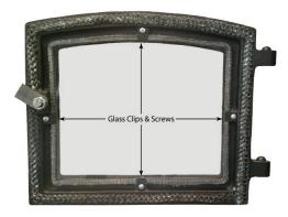
**REPLACING CERAMIC GLASS:** Never operate the wood heater with damaged or broken ceramic glass. Never substitute window glass or tempered glass as a fire may result. Replacement 5mm high temperature ceramic, complete with gasket, is available from your dealer. (P/N GLS1300)
