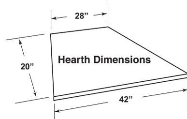
Framing dimensions in illustrations accommodate 1/2" finishing material.
