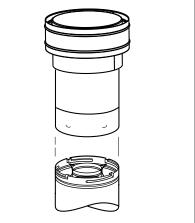
Figure 34: Attaching Vertical Termination
