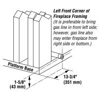
Figure 17: Routing Gas-line
