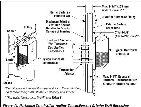
NOTE: The horizontal termination must not be recessed into the exterior wall or siding by more than 1-1/4" (32 mm), as shown in *Figure 41*.
