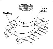
Figure 33: Installing Storm Collar
