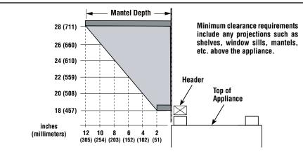
Figure 2: Minimum Clearances to Combustible Mantel
