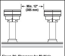
*Figure 31: Clearance for Multiple Vertical Vent Terminations*
