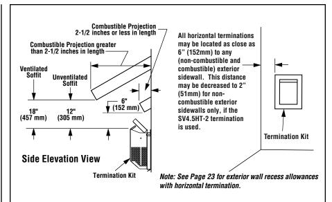
Figure 38: Horizontal Termination Clearances
