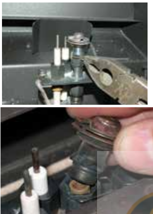
Remove the 2 screws, push Burner Assembly to the left and lift out.
