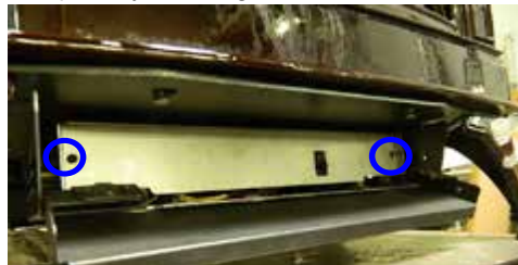
Take the valve cover plate out
