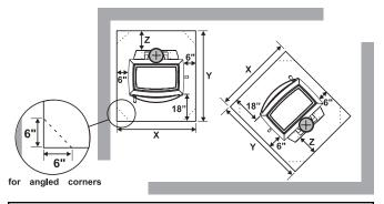
NOTE: In Canada, floor protection must extend 18" to the front and 8" to each side of the stove.
