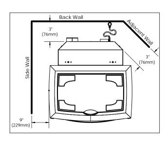
These dimensions are minimum clearances but it is recommended that you ensure sufficient room for servicing, routine cleaning and maintenance.
