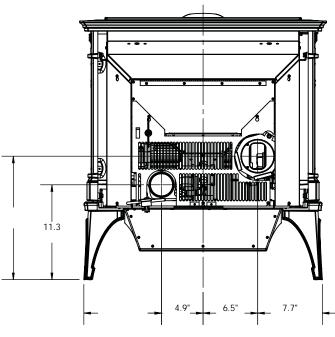
This unit uses a 4" exhaust vent.
