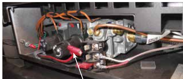
Diagram 3 - Red TH wire disconnected
