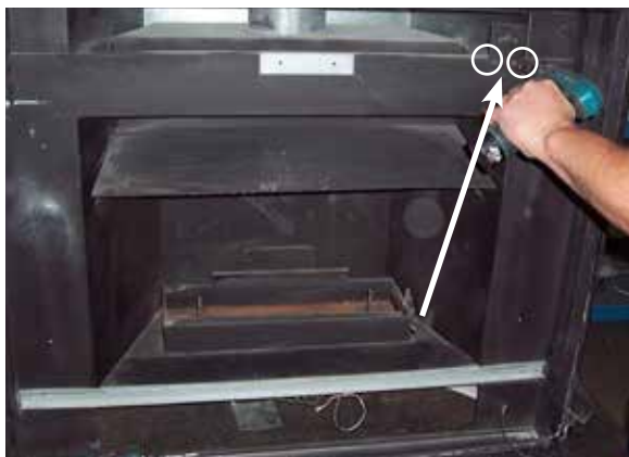
Remove 2 screws - remove Thermodisc Bracket
