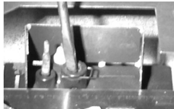
**Step 4.** Pull the pilot cap straight up to remove and expose the pilot orifice.
