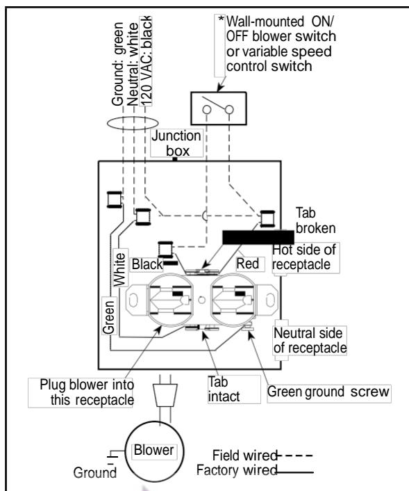
**Figure 33: Wiring Diagram—Millivolt Gas Valves**
