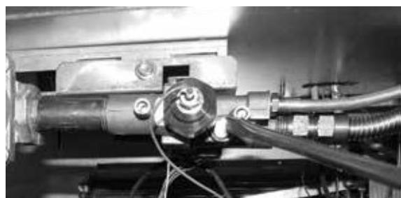
**Step 1.** Remove Burner assembly and replace the main orifice supplied in Kit.
