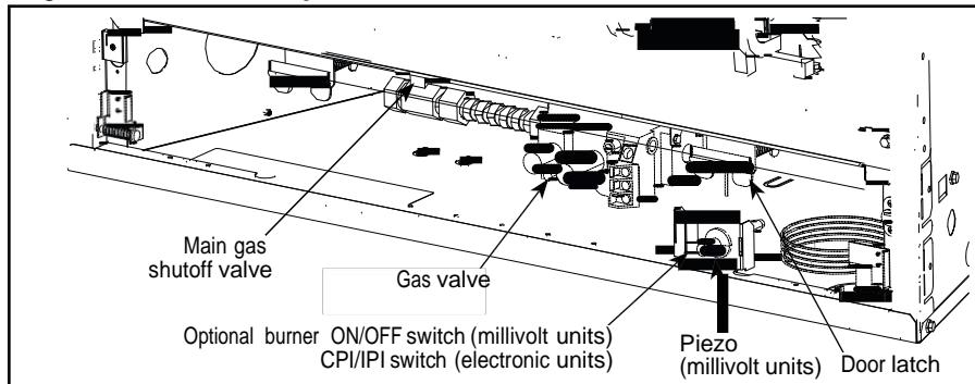
**Figure 35: Gas Line Connection**
