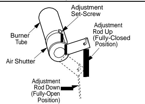
1. Move the adjustment rod down to increase air flow and up to decrease it. The rod is located in the lower control compartment. Position the air shutter to the factory setting (**Table 29**).
