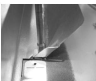
**Step 2:** Secure all three of the screws to the up-right positioned heat shield - one (1) at both ends and one (1) in the center.
