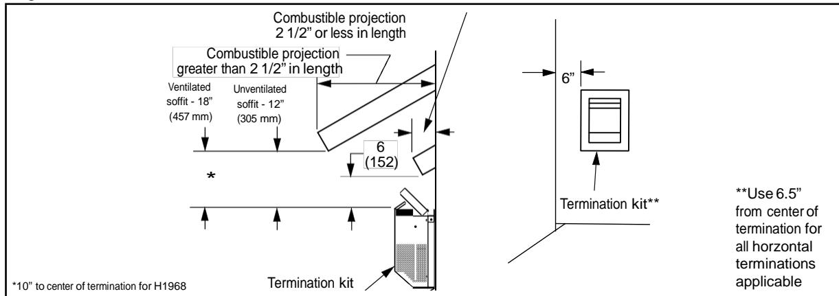
**Table 7: Horizontal vent termination clearances for buildings with combustible and noncombustible exteriors**
