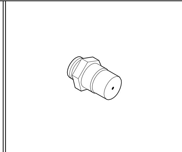
12. Use pipe joint compound or Teflon® tape on all pipe fittings before installing.
