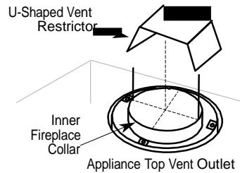
**Figure 14: Vent restrictor installation, Rear vent**
