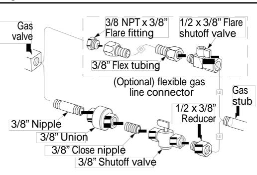
These fireplaces are equipped with a gas flex line for use (where permitted) in connecting the unit to the gas line. A gas flex line is provided to aid in attaching the direct-vent fireplace to the gas supply. The gas flex line can only be used where local codes permit. The flex line is rated for both natural and propane gas. A manual shut off valve is also provided with the flex line.
