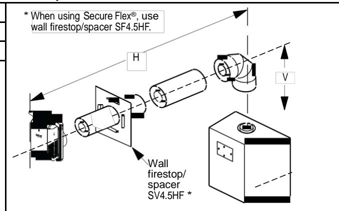
**Table 23: Top Vent—One 90° Elbow, Elbow Connection NOT at Fireplace**
