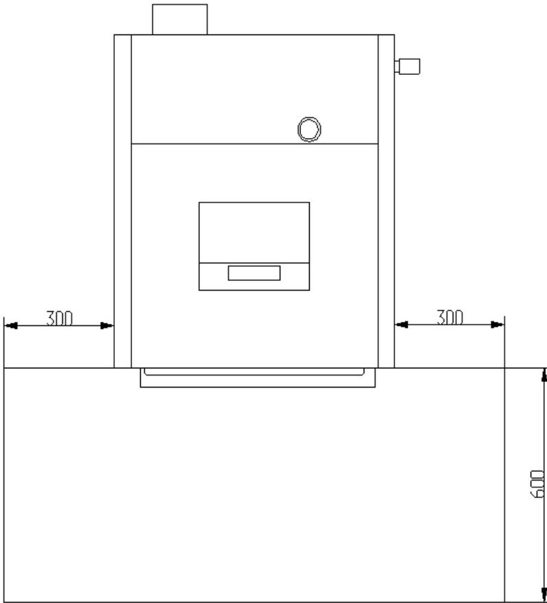
**Recommended clearances for BM 25,40,60,80 (in mm)**
